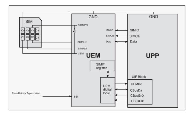
The internal clock frequency from UPP CTSI block is 13 MHz in GSM. Thus to achieve the minimum starting SIMCardClk rate of 3.25 MHz (as is required by the authentication procedure and the duty cycle requirement of between 40% and 60%) then the slowest possible clock supplied to the SIM has to be in the GSM system clock rate of 13/4 MHz.
