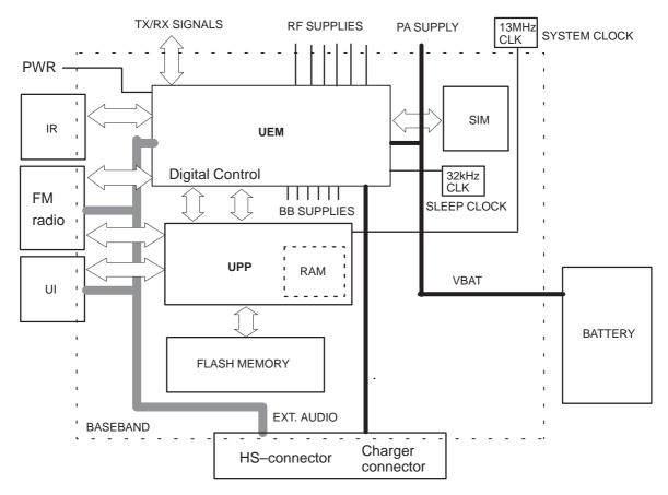
UPP ASIC (Universal Phone Processor) provides the MCU, DSP, external memory interface and digital control functions. UEM ASIC (Universal Energy Management) contains power supply circuitry, charging, audio processing and RF control hardware.
