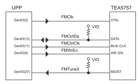
NOTE: *FMCtrlClk* needs to be set to logic '1' when data is not written or read. This is required for correct operation of the *FMTuneX* signal.
